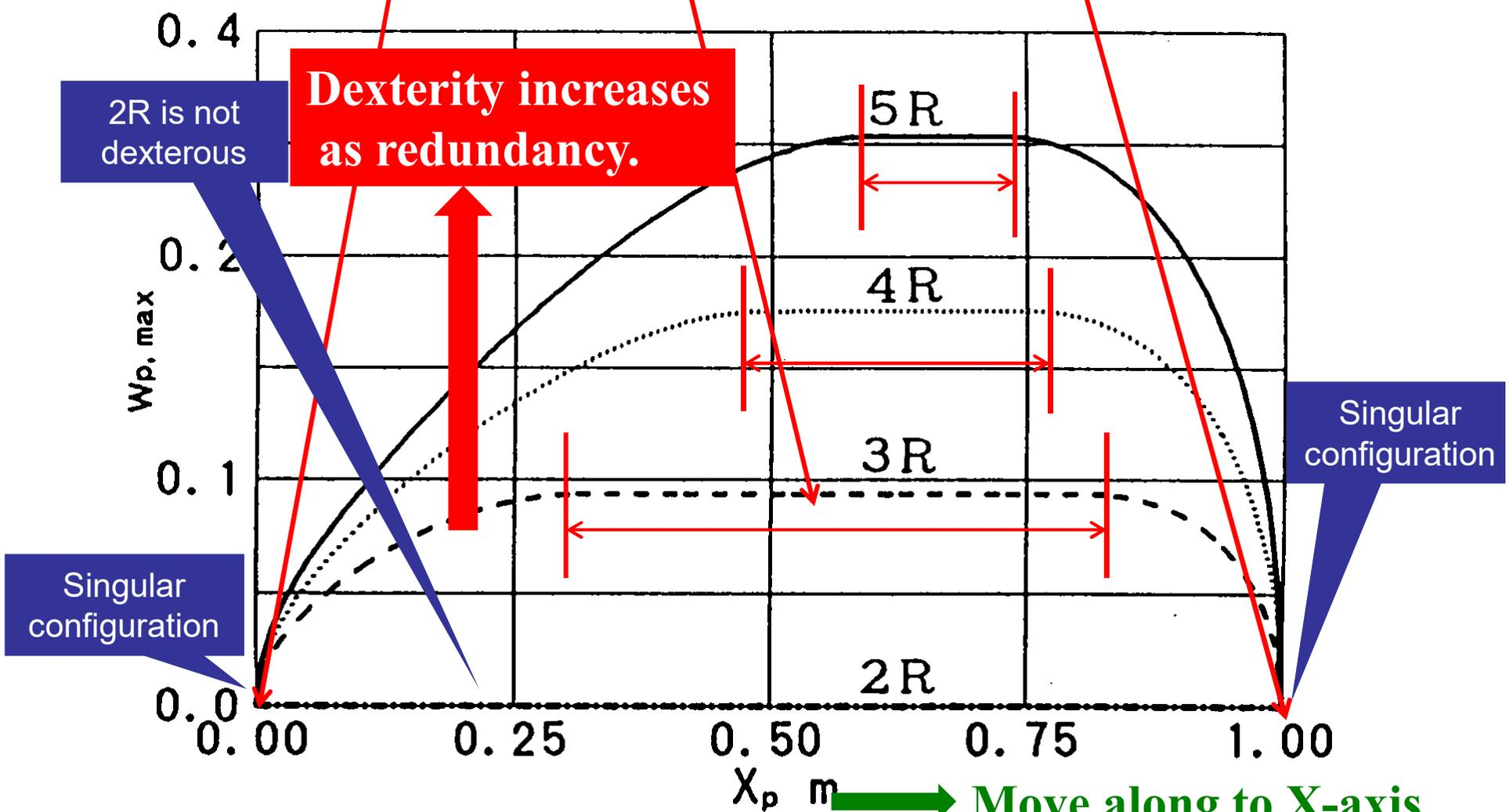
The maximum manipulability measure of serial planar manipulators
