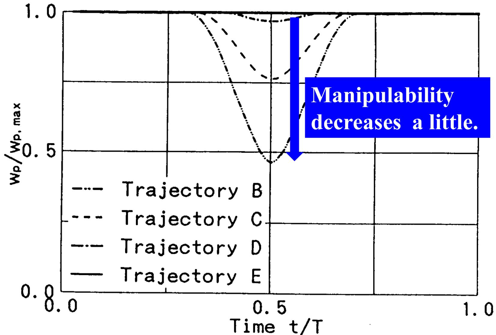
**Manipulability measure in the optimum CP control in case where posture angle of end-effector is continuously specified (4R-manipulator)**
