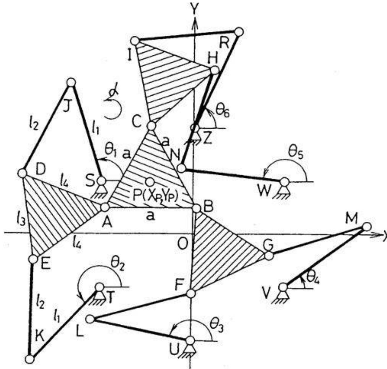
A **Redundant** closed-loop planar manipulator with 6 DOF
