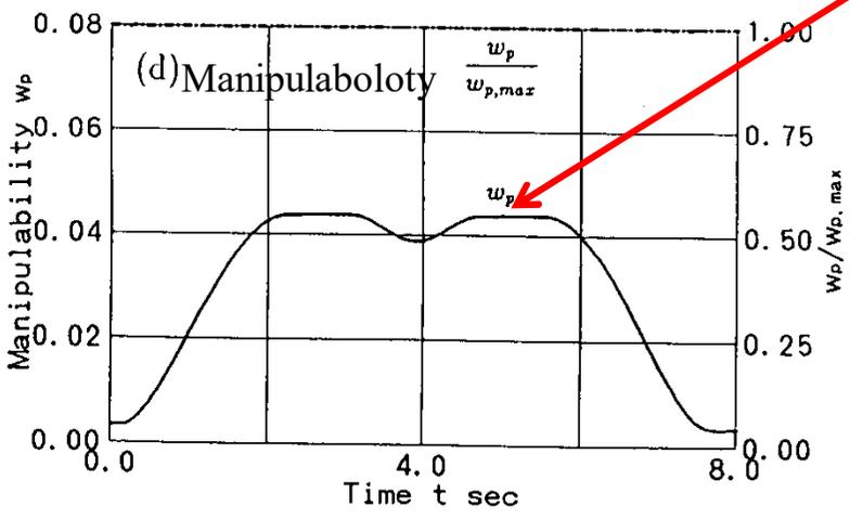
**Result of the optimum CP control (4R, trajectory B)**
