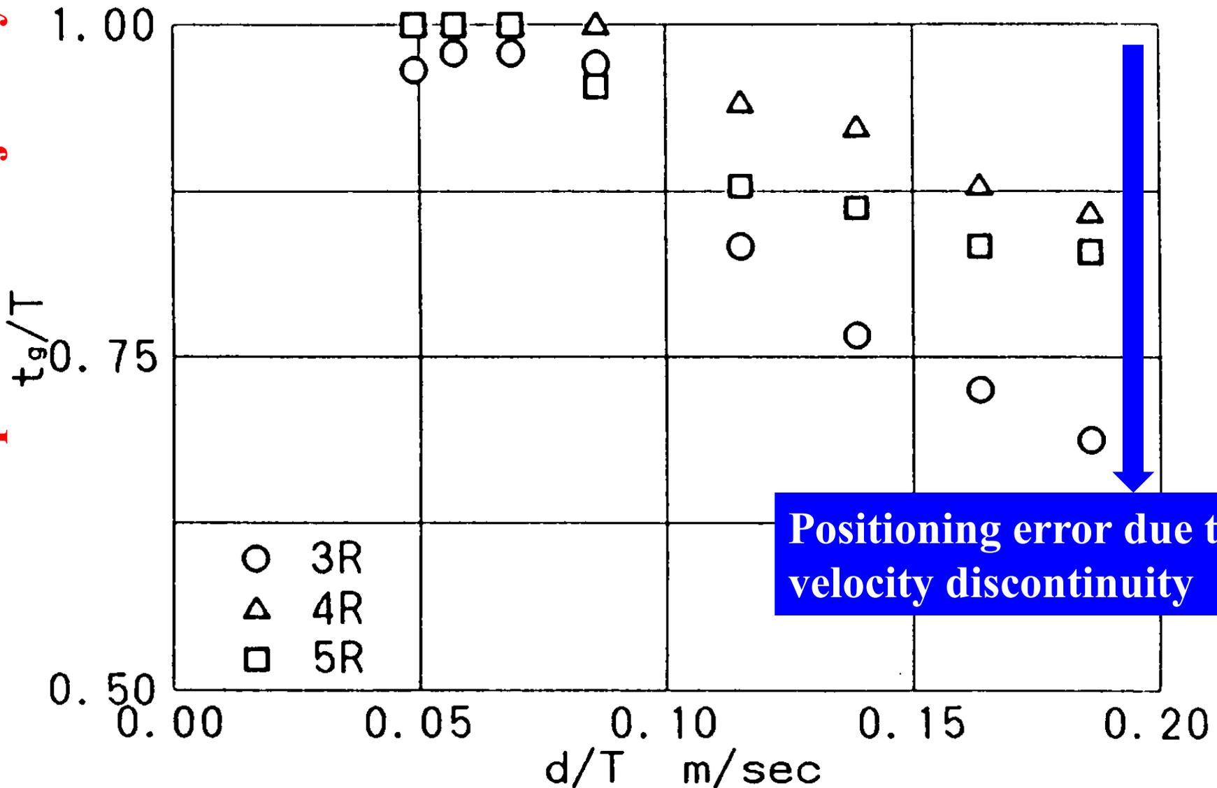
**Positioning error due to velocity discontinuity**
