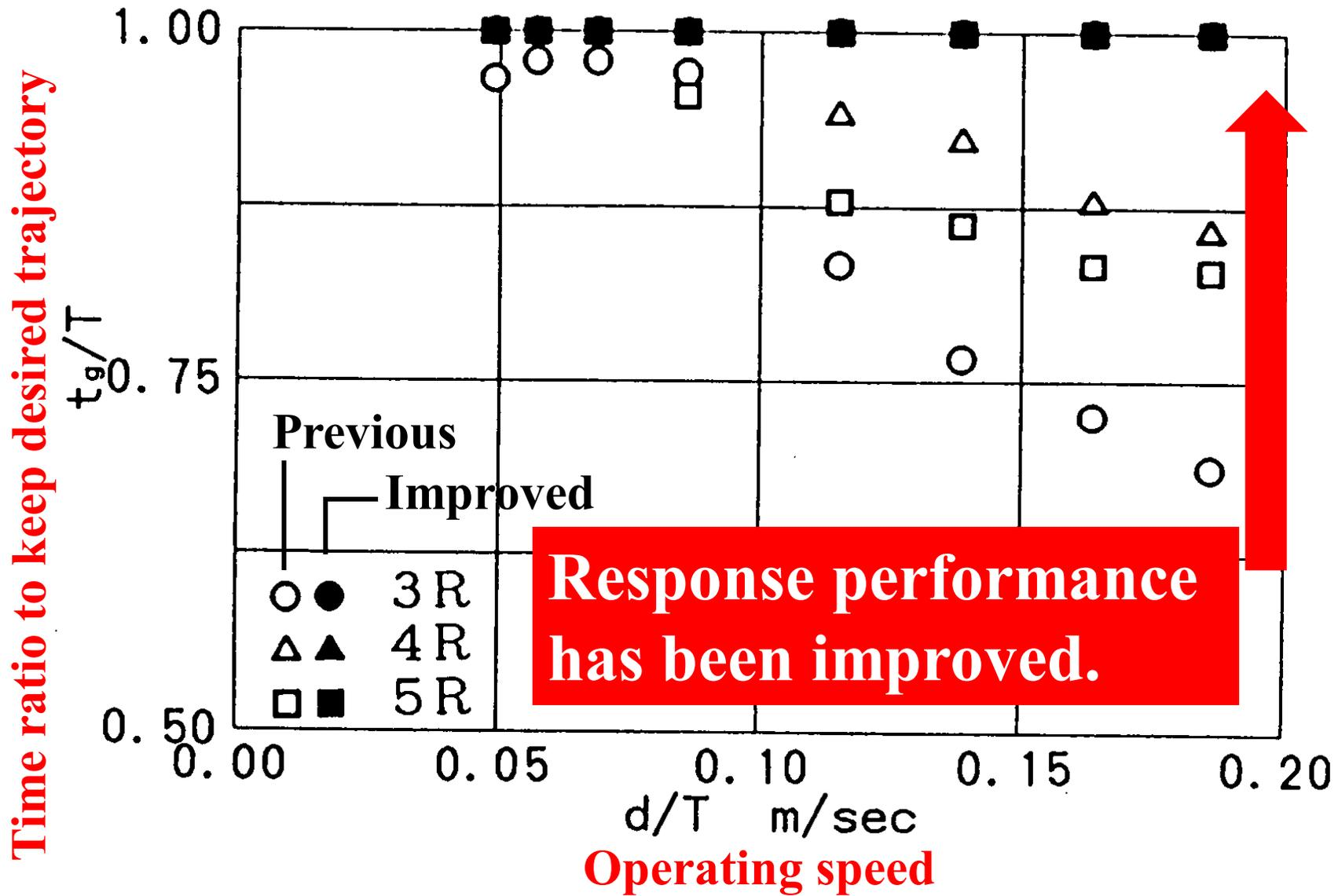
**Performance on response in the optimum CP control in case where posture angle of end-effector is continuously specified (various manipulator)**
