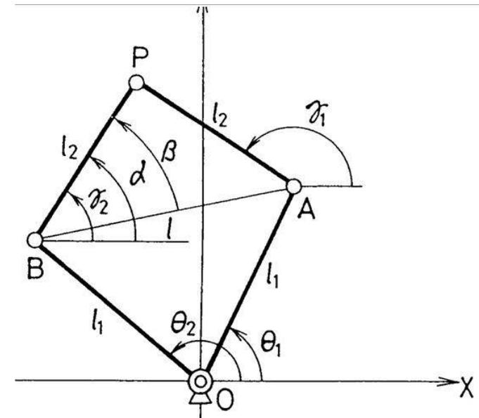
Ex. Planar closed-loop mechanism with 2 DOF
